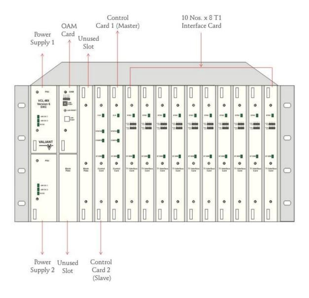
The equipment provides a wide choice of access ports for connecting to and executing management and configuration commands through its OAM Card.
