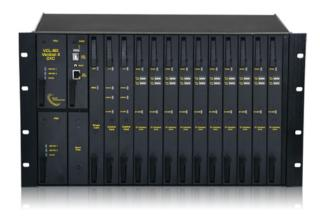
This product offers 1+1 -48V DC Power Supply Redundancy, 1+1 Control Card and Processor Redundancy, 1+1 Cross-Connect (TSI) Redundancy, 1+1 Timing (Synchronization Clock Circuitry) Redundancy. This DXC offers "user selectable" clock / timing synchronization priority. The Dual Power Inputs allow the equipment to be powered from two separate power sources. AC input external adapter is an optional for AC mains operation.
