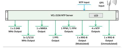
The VCL-2156 is equipped with a highly accurate, low-noise OCXO to provide a high stability, ITU-T G.812, Type II, III compliant holdover clock with better than 12µs accuracy over a 24 hour (5 milliseconds per year) period in the event of unavailability of the GPS / GNSS signal, or GPS / GNSS antenna failure, or a temporary loss of reception in a totally isolated network without any external
